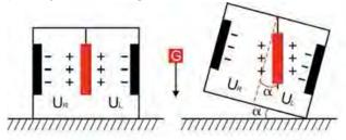
$U_{R_s}$ ,  $U_L$ Respectively is the pendulum left plate and the right plate corresponding to their respective voltage between theelectrodes, when the tilt sensor is tilted,  $U_R$ ,  $U_L$  Will change according to certain rules, so  $f(U_R, U_L)$  On the inclination of  $\alpha$  function:
